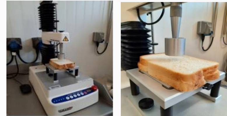
Figure 4.4. a) Texture Analyzer (TA.XT Plus, Stable Micro System, UK); b) 35 mm probe
